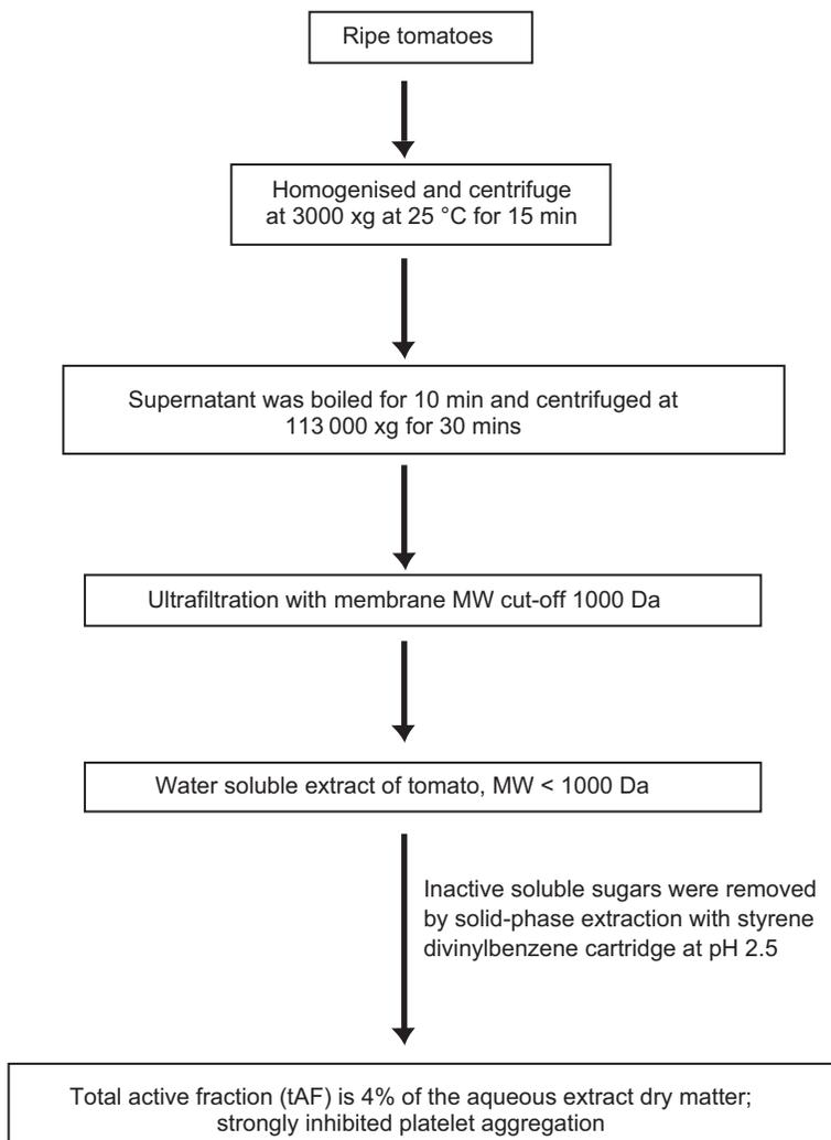
Fig. 5.2 Outline of water-soluble tomato concentrate preparation. Adapted from Dutta-Roy *et al.* (2001) and O’Kennedy *et al.* (2006a).
